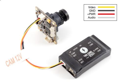
A pilot camera can be installed on the CAM port. The port has input for both video and audio - if external audio jumper is enabled inside the unit. An external microphone can be connected to the white (audio) and black (-) wires.
