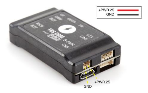
The backup power port is selected when the voltage of the main battery is lower than the backup battery. To add backup power to the system, connect an 2S (7.4V) battery (max. allowed) to the B-PWR port using a 2-pin Molex PicoBlade 1.25 cable (available separately).
