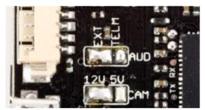
The TBS CORE PNP PRO has no on-board microphone to keep the size down, but can still be connected externally via the CAM-port.
