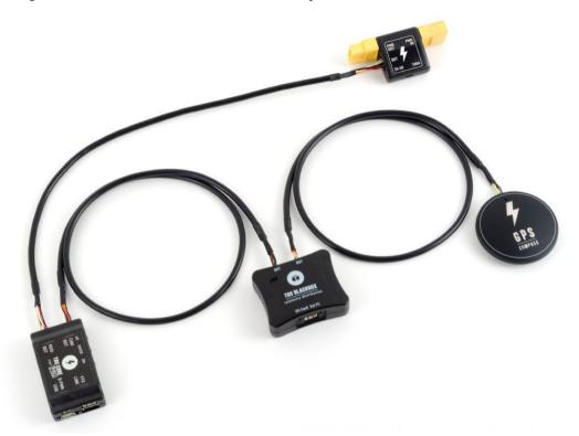
Pick a suitable length BST cable for your setup and connect the TBS GPS/COMPASS module to any BST port on either the BLACKBOX or CORE PRO unit (shared bus).
