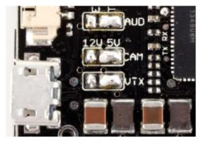
Important: when using video transmitters with on-board voltage regulators (e.g. IMRC VTx), it is recommended to connect the positive and ground lead directly to the main power leads instead to maintain good switching efficiency and stability.
