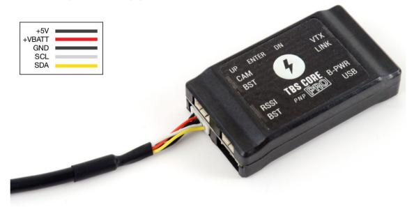
There are two BST (I2C) ports on the left side of the unit. These can be used to connect a range of compatible modules for the TBS CORE PNP PRO to provide telemetry data. This modular system allows you to custom fit your model depending on your exact needs and weight budget. This is a shared bus, meaning all BST ports use the same physical communication lines. The pin-out is the same for all BST modules.
