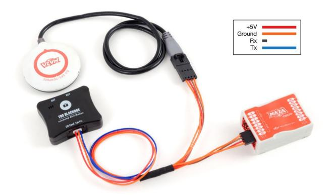
The BLACKBOX (available separately) acts as a central recipient for telemetry data from the TBS Current Sensor, TBS GPS/COMPASS, or DJI NAZA flight control. It forwards that information to the TBS CORE PRO live OSD and continuously logs it all on a SD card. This makes keeping a flight logbook easy.
