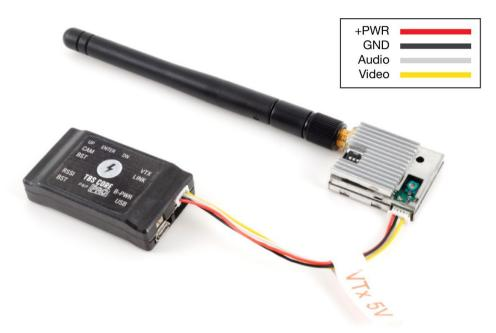
A video transmitter can be installed on the VTX port. The TBS CORE PNP PRO can power any video transmitter up to 1W. You can customize the included cable to suite your particular VTx, but be cautious of the voltage selection and wire polarity.
