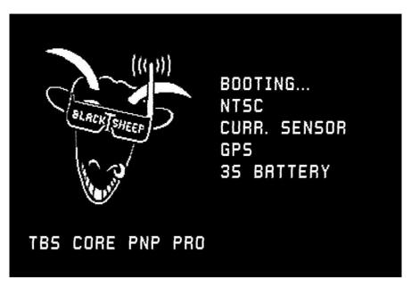
When power is supplied to the system, a boot screen will display detected the video format (NTSC/PAL), any connected BST modules and the battery type (2S-6S). The battery type detection is only available if the voltage warning is set to Auto.
