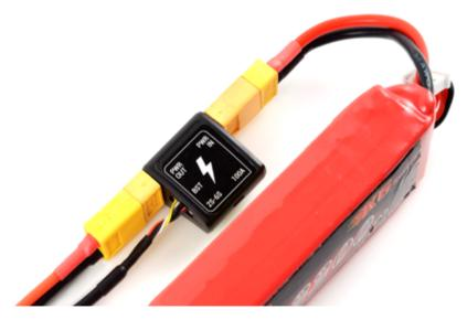
The current sensor comes with a protective plastic casing (the photo above is from the prototype). It is rated for maximum 100A, which should cover even the biggest aircrafts. The sensor's digital interface provides the most accurate current sensing yet. A blue light indicates on the front of the casing shows that battery power is connected. In addition to current sensing, it supplies power to the main CORE processing unit.
