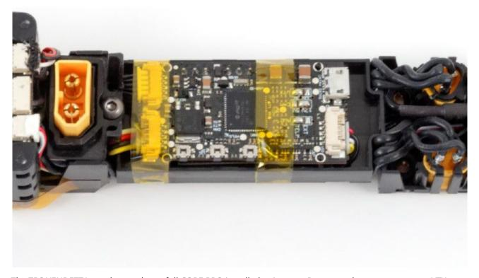
The TBS VENDETTA quadcopter has a full CORE PRO installed at its core. It powers the system camera, VTX and BST line, establishes the link to the TBS COLIBRI RACE flight controller, displays/manages the stick-navigation of the OSD, and performs the SmartAudio configuration of the UNIFY PRO 5G8 VTX.
