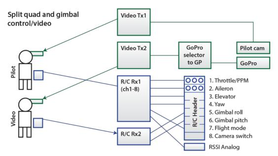
• **Dual operator with yaw authority** - To give the video operator the ultimate freedom over framing and picture positioning, swap the responsibility for yaw control over to the the video operator. This requires good piloting skills and continuous communications back and forth to practice safe maneuvering and flight.
