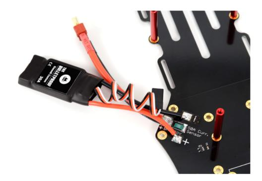
One important note for ESCs that do not carry the "OPTO" label or are not TBS BULLETPROOF designs, is that only one of the four ESCs should provide 5V BEC power to the flight controller. The middle red wire on the end connector should be disconnected on three of the ESCs. If the flight controller is providing power (e.g. NAZA-M PMU/V-SEN-unit), all ESC BECs should be disconnected. The reason for this is to avoid voltage oscillations caused by erroneous voltage-regulator feedback.
