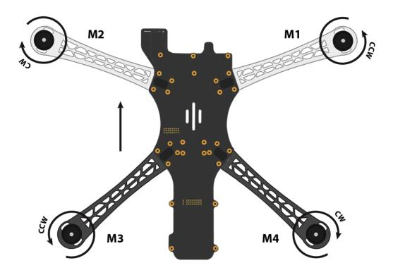
• Plug in the bullet-connectors to the speed controllers. Swap any two wires to change the direction of rotation if they do not rotate as shown below. See the image above for the most commonly used motor setup (e.g. NAZA-M.)
