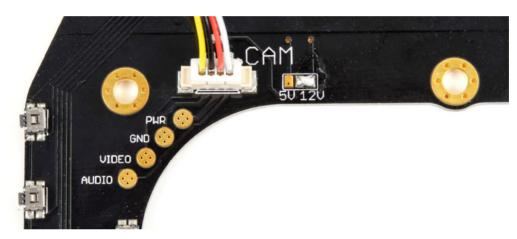
• Plug in the cable connector for the camera and insert the tabs on the top and bottom of the camera frame in the corresponding routed gaps on the frame. For a secure mount, you can add solder to the three exposed solder spots, or leave it for easy hot swapping in the field.
