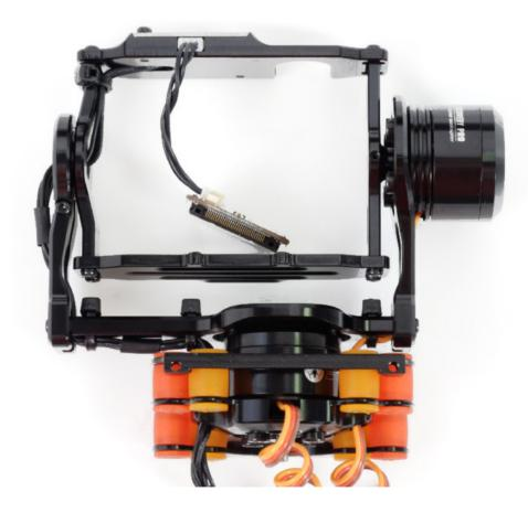
• Next, put the bearing into the housing the left gimbal arm and use the long M2x12mm screw to compress the gap until the bearing stays in place - do not overtighten, just clamp the bearing.
