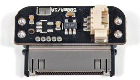
(Advanced users only) There is even a component you can add on the board to be able to change the charging rate from 1A to 0.5A continuous. To reduce the charging rate, order the IC part NCP380HSN05AAT1G from Mouser or Digi-Key and solder the IC to the unoccupied pads on the adaptor board (adequate soldering skills needed.)
