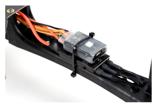
• Feed the battery straps through the two slots in the battery compartment. Only one strap is really necessary to provide adequate friction to keep the battery fastened.
