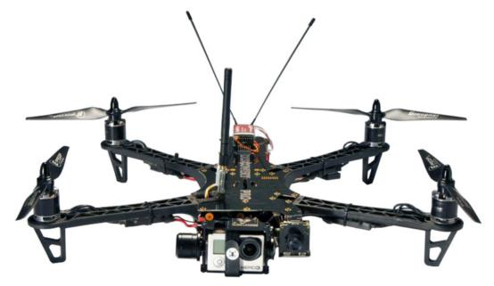
By implementing the wiring into the frame, the copter is easy to build and outperforms similar quads in terms of FPV range and video link quality. The DJI Flamewheel arms as predetermined breaking point protect your electronics and are easily replaceable in the field.
