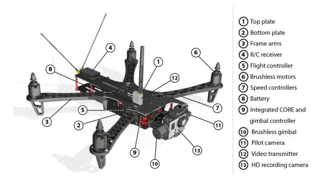
Before adding the equipment to the frame it is a good idea to become familiar with the recommended positioning of the equipment, as shown in the image above.
