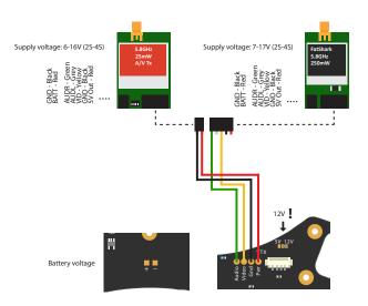
**Note:** Connecting a video transmitter directly to a shared battery source may induce interference on the video image. Consider adding a filter between the solder pad and video transmitter.
