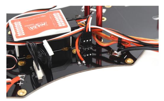
• (DJI NAZA only) To save weight and space, the PMU (V2) can be disconnected and removed after the final configuration has been made. Although, 5V power still has to be provided from at least one of the ESCs.
