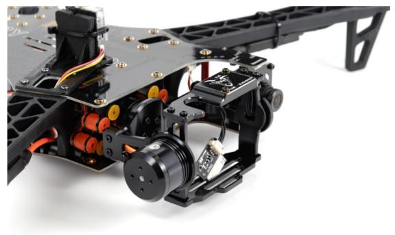
**Important:** Avoid rotating the gimbal multiple full turns on the tilt-axis. This puts tension on the IMU cable which in turn introduces counter-forces and interferes with the normal operation of the gimbal.
