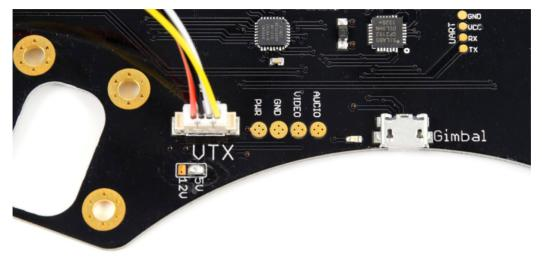
• The kit includes a small JST cable which is compatible with Lawmate 500mW VTx as well as our TBS GREENHORN and TBS ROOKIE. For FatShark VTx you need to cut the cable and solder your FatShark cable onto it. The connector wire color and signal arrangement is shown in the picture above.
