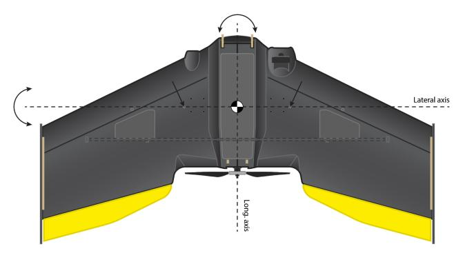
Balance the lateral (pitch) axis within the recommended CG spot. The longitudinal (roll) axis should be balanced straight along the middle of the wing.
