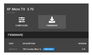
Update your CROSSFIRE/ TRACER TX to FW 3.71 (or later) by Agent X. If you can't see the required FW version, click on the 3 dots in the top right corner and check "include beta releases".
