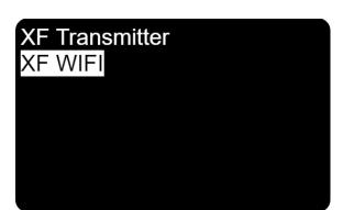
Connect your CROSSFIRE/ TRACER to the internet via the built-in WiFi module. You can provide access point information from your nearest wifi hotspot, or create a temporary one on your phone. Wait for it to switch to "Online" under XF WIFI/ About
