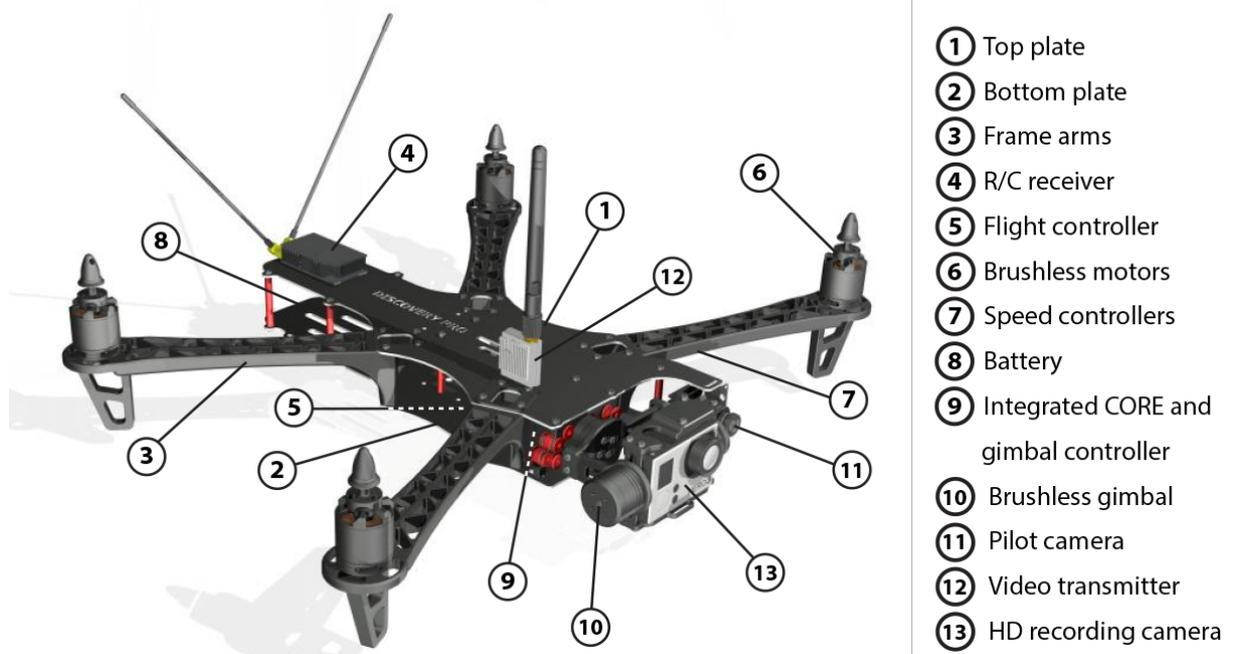
Before adding the equipment to the frame it is a good idea to become familiar with the recommended positioning of the equipment, as shown in the image above.
