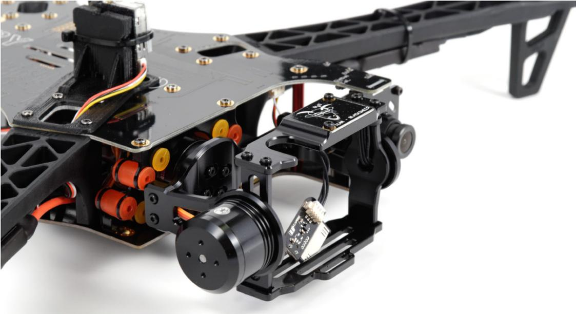
**Important:** Avoid rotating the gimbal multiple full turns on the tilt-axis. This puts tension on the IMU cable which in turn introduces counter-forces and interferes with the normal operation of the gimbal.
