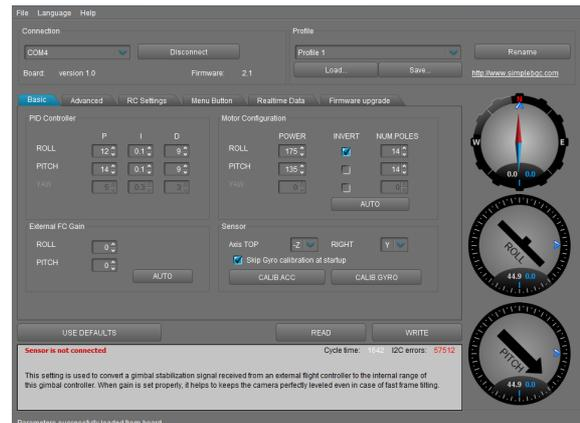
DISCOVERY PRO utilizes two profiles, one silent profile (Profile 1), to keep the gimbal quiet while on ground and one noisy profile (Profile 2). The CORE MCU will detect when main motor starts (current consumption >3A) and switch from the silent to noisy profile automatically. If you change something in SimpleBGC you have to **do the change on both profiles**. If you want to change your in-flight values you have to do this on Profile 2.
