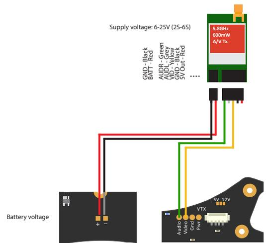
**Note:** Connecting a video transmitter directly to a shared battery source may induce interference on the video image. Consider adding a filter between the solder pad and video transmitter.
