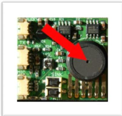
A clean, well thought out installation is critical to providing the greatest accuracy possible. A good place to put your Variometer is embedded in the wing or below the battery in the fuselage. You can cover the Variometer with packing sponge to even further increase its accuracy. While it is not recommended to shrink-wrap your Variometer as it can be damaged in the process, it is certainly possible to do so. Make sure you do not cover the round hole of the pressure sensor.
