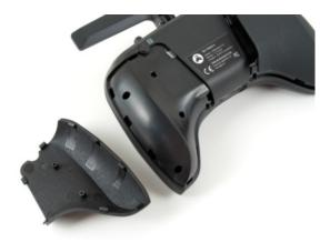
Then remove the six (6) screws, as indicated in the following photo with an M1.5 hex driver. Now, the back housing lifts off.
