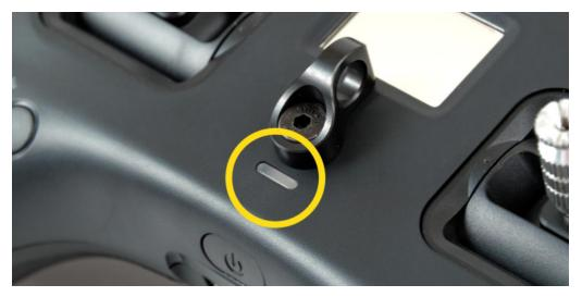
When the remote is powered on, the LED behind the button will show the actual status of the remote. The built-in LiPo battery is charged every time a 5V power source is connected to the USB-C connector.
